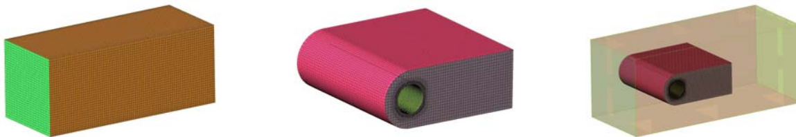
Fig. 2. 2D cylinder case: background mesh (left), moving mesh (middle) and overlapping region (right)
